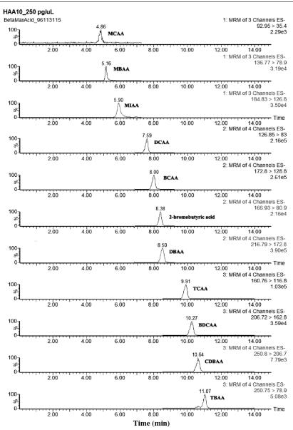
**Figure 1.** The chromatogram of HAAs on BetaMax Acid column (individual HAA concentration was 250 pg/ $\mu$ L, injection 50  $\mu$ L).
